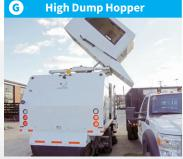
Variable dump height hopper (up to 11' high) with 44" extra-long dump door easily reaches most dump trucks.
