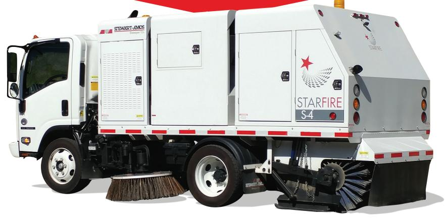
An *Effectively Simple*, Full-Featured, Heavy Duty 4 yd<sup>3</sup> Broom Sweeper Mounted on a Highly-Maneuverable, Non-CDL Chassis
