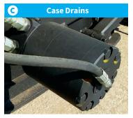
Case drains for all the hydraulic motors protect shaft seals from pressure leaks, minimizing repairs & replacements.
