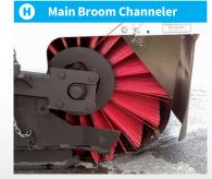
Main broom channeler (optional) effectively sweeps large quantities or bulky & light debris (leaves/pine straw). Self-adjusting as main broom wears.
