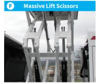
Massive double "X" style lift scissors & 4-corner hopper lift ensure exceptional hopper stability when dumping wet, unbalanced, or sticky debris.
