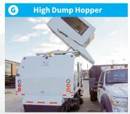
Variable dump height hopper (up to 12' high) with 44" extra-long dump door easily reaches most dump trucks.
