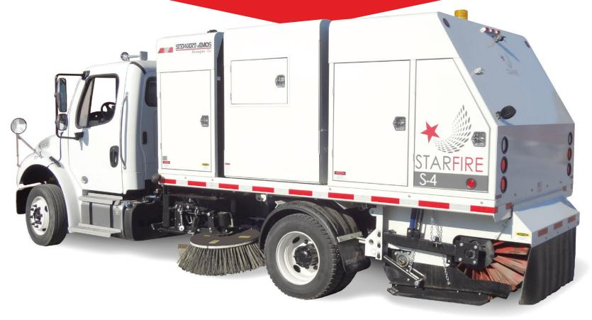
An *Effectively Simple*, Full-Featured 4.5 yd<sup>3</sup> Mechanical Broom Sweeper Mounted on a Large, Non-CDL Chassis
