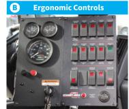
Vertically-mounted control panel is 6-way adjustable for easy & ergonomic viewing. One-touch sweeping allows for operator to preset functions. Brooms raise automatically in reverse.
