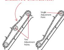
Extended Chain Life. 3rd shaft provides proper return (upper) chain support. This allows chains to run as loose as possible, dramatically improving chain wear life versus similar 2-shaft designs.
