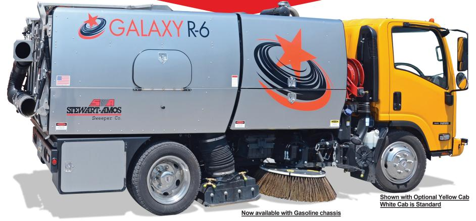
An *Effectively Simple*, 6 yd<sup>3</sup> Regenerative Air Street Sweeper Mounted on a Highly Maneuverable, Non-CDL Cab-Over Chassis
