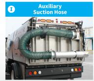
Optional 10' Auxiliary Suction Hose with 4' aluminum tube helps clean storm drains.
