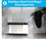
Stainless steel, centrifugal dust separator located inside the hopper separates fines from the air stream.
