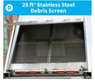
28 ft² stainless steel debris separator screens maximize sweeping productivity. Screens can be easily cleaned from outside of unit. Bolt-in design makes screen replacement easy.
