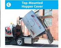
The top-mounted hopper cover opens automatically during dumping cycle to provide quicker, easier & safer cleaning of stainless steel screens & hopper.
