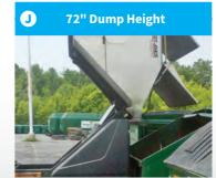
Rear 72" dump allows for convenient on-site disposal into 5'+ dumpsters. Exclusive 3" hopper slide-back feature moves hopper rear-ward allowing it to clear dumpster edges.
