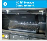
Large, one-piece polyethylene storage compartment provides nearly 80 ft³ of space for tools, tires, etc. Compartments are lockable and are illuminated with 2 LED lights
