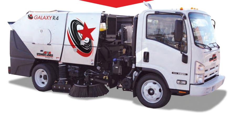
An *Effectively Simple*, Full-Featured, High-Dumping Regenerative Air Street Sweeper Mounted on a Highly Maneuverable, Non-CDL Cab-Over Chassis
