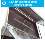
14.4 ft² stainless steel debris separator screens maximize sweeping productivity. Screens can be easily cleaned from outside of unit. Bolt-in design makes screen replacement easy.
