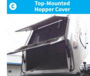
The top-mounted hopper cover opens automatically during dump cycles to provide quicker, easier & safer cleaning of stainless steel screens & hopper.
