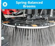
Spring-balanced, free-floating gutter brooms automatically apply correct surface pressure for maximum broom wear life.
